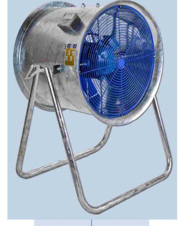
inlet and discharge epoxy coated guards, to prevent heavy air borne particles going through the unit. They further protect the user from accidental contact with the rotating impeller whilst the fan is running. An IP55 rated external terminal box is fixed to the fan casing to simplify the electrical connection to the fan motor. A starter or isolator with a requested length of PVC cabtvre, can also be fitted onto the external fan casing on request. The complete fan
